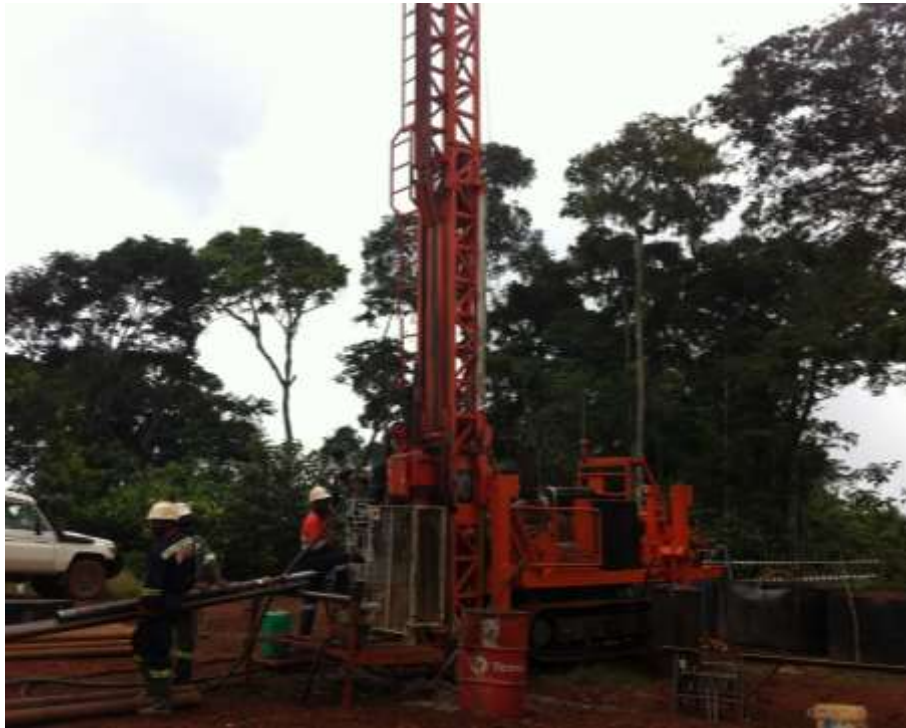
Figure 5 –Drilling at Nabeba, using one of the Company’s four drill rigs (2 Diamond, 2 RC)
