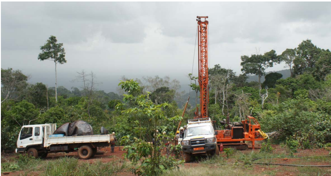
Figure 8 – Sundance Diamond Core Rig operating at Nabeba
