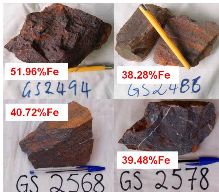
Figure 5 - Grab Samples from Ntam (Mbarga) with Niton Fe Values Greater than 35% Fe
